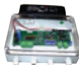
PWM driver for fixtures with autonomous colour programs for stand-alone or controlled working by means of DMX 512 protocol for installations of all sizes.
